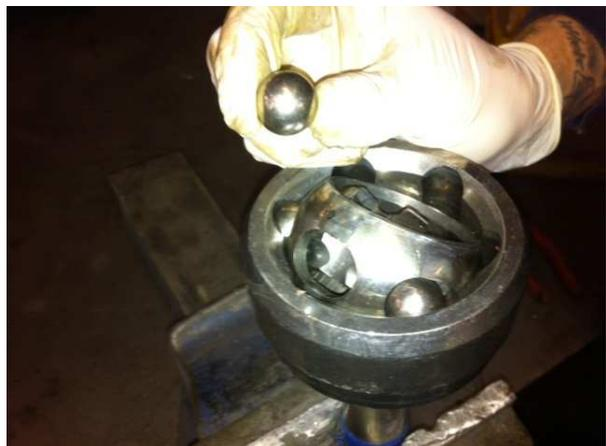
Move around the cv working in opposites until all the ball bearings are removed.
