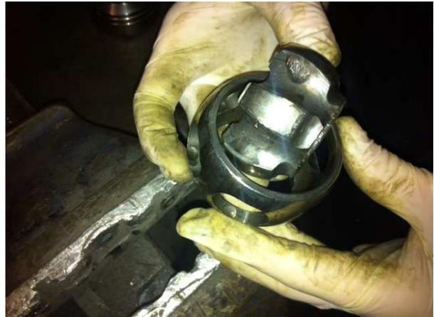
(The bottom of the cage is the end with the larger inner opening and closest to the openings where the ball bearings locate, the top of the spider inner is recognised by the flats on the ends of the lands.)
