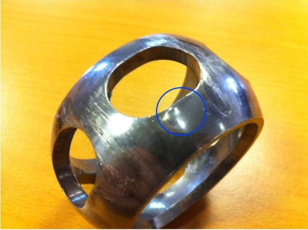
Use a die grinder with a metal cutting tool to remove the high spots and to restore the components to their original shape, test fit the components together and check for ease of movement. The components should move smoothly and not bind tight.
