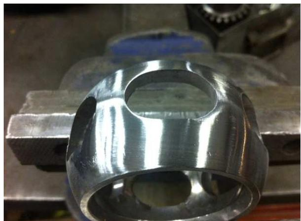
Fill the CV with K48 Moly grease and refit to vehicle.
