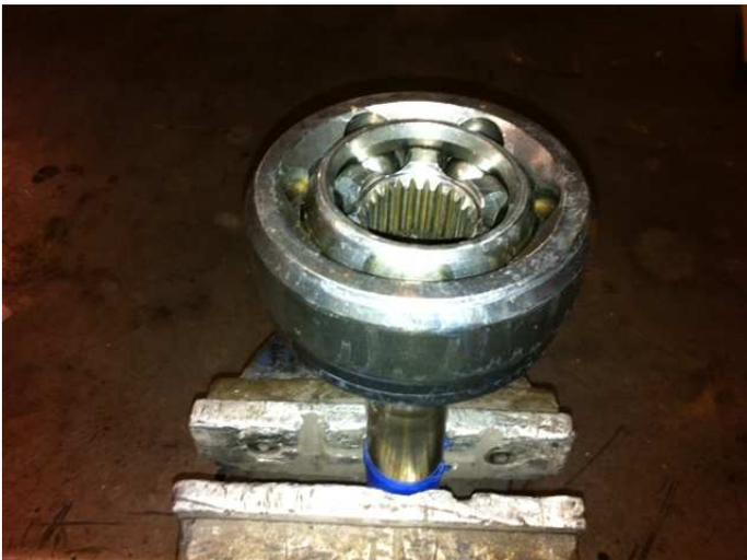
To remove the ball bearings use a soft punch (aluminium) and a hammer and strike down on the outer cage directly above a singular ball bearing location. With some persuasion the ball bearing opposite to this location will rise to its highest point and come free from the cage, remove the ball bearing and repeat the striking process on the opposite ball bearing location.
