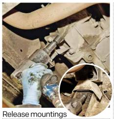
Undo the four 15mm bolts securing the bracket to the transfer box. Remove the nut on the nearside mount's stud; don't unbolt the bracket as it's attached to the gearbox rather than the transfer box. This allows enough movement for the assembly to be jacked up.
